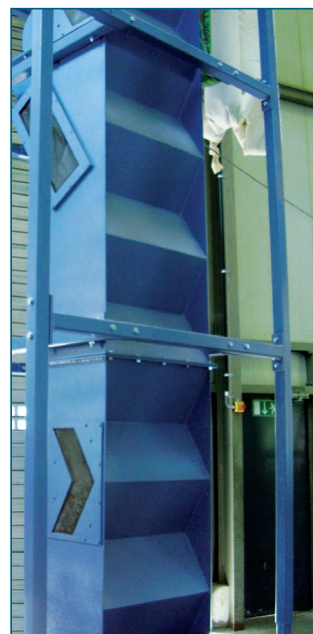
Fig. 2: Channel of an air stream separator
