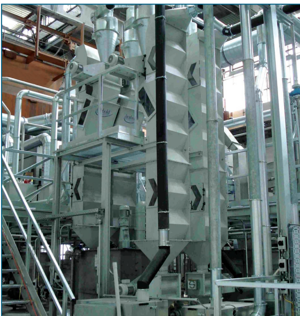
Fig. 1: Herbold air stream separator in a PET bottle washing line
