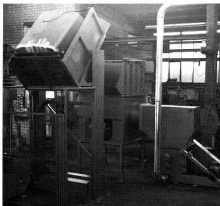
Central granulator for the reduction of sprues
