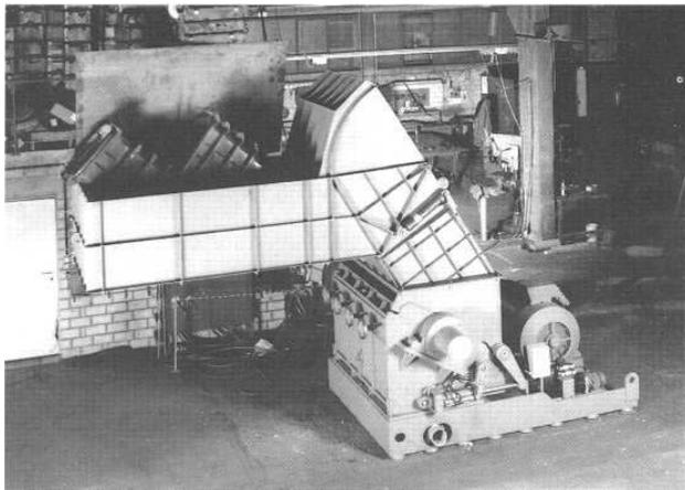
HERBOLD has developed a new type of feed device which solves these problems in a surprisingly simple manner. The material, fed in bundles is separated and fed into the granulator in portions. The grinding chamber is hermetically enclosed as soon as the feeding process commences.
