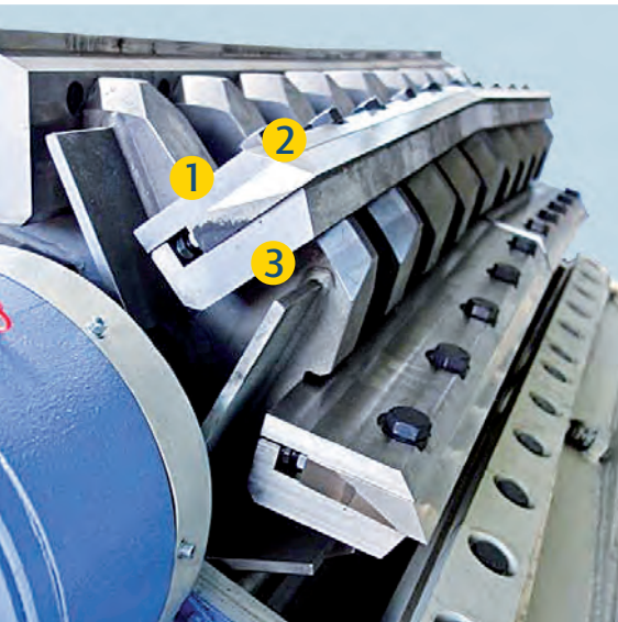
Rotor type F with exchangeable wear protection
