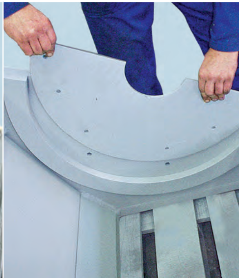
Housing with exchangeable armour plating
